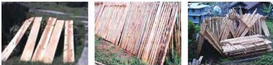
Plate 19. Drying lumber under the sun
