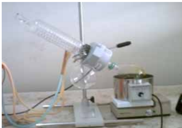
C. Rotary Evaporator (concentration of solutions under vacuo )
