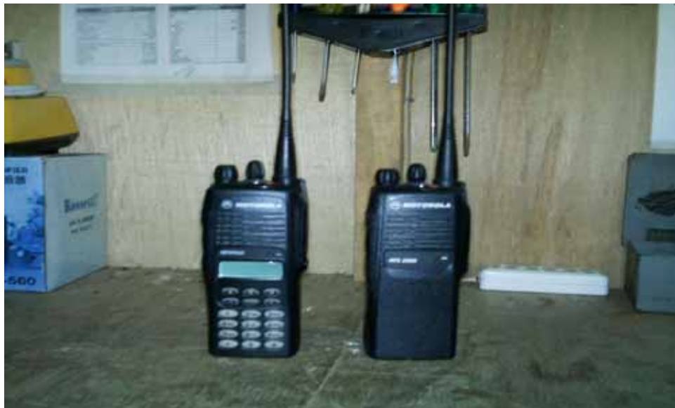
Plate 3. MOTOROLA ATS 2500 Handheld Radio (UHF)
