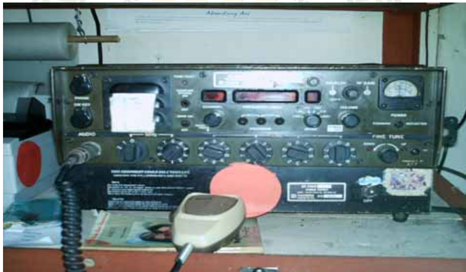
Plate 6. Harris 100 W Transceiver (HF SSB)
