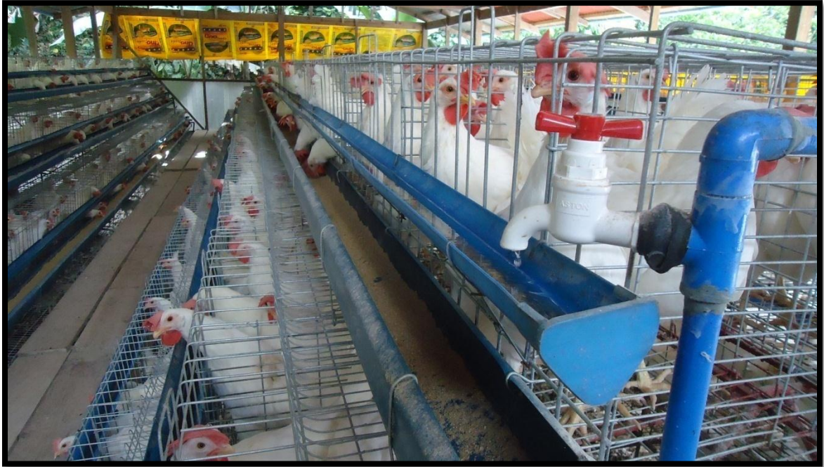
Figure 7. Plastic pipes for providing water
