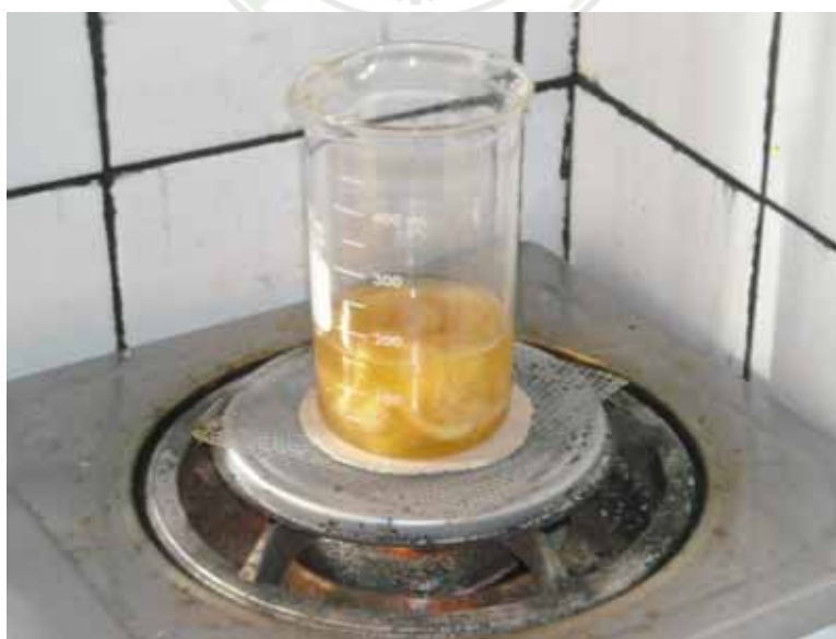
Figure 28. The extracted dye with the raw silk is in the beaker being heated
