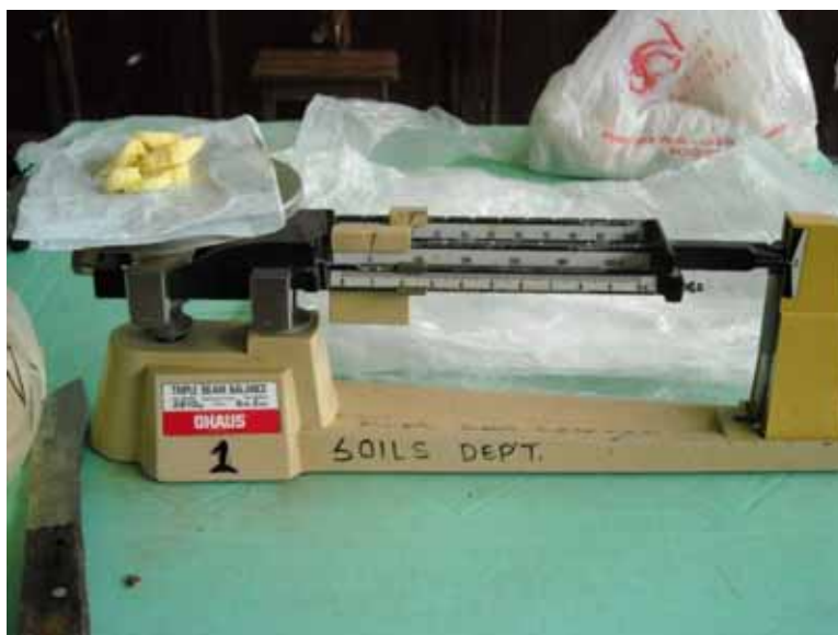
Figure 21. Weighing the 20 grams root flesh in the triple beam balance at the Soils Science Laboratory
