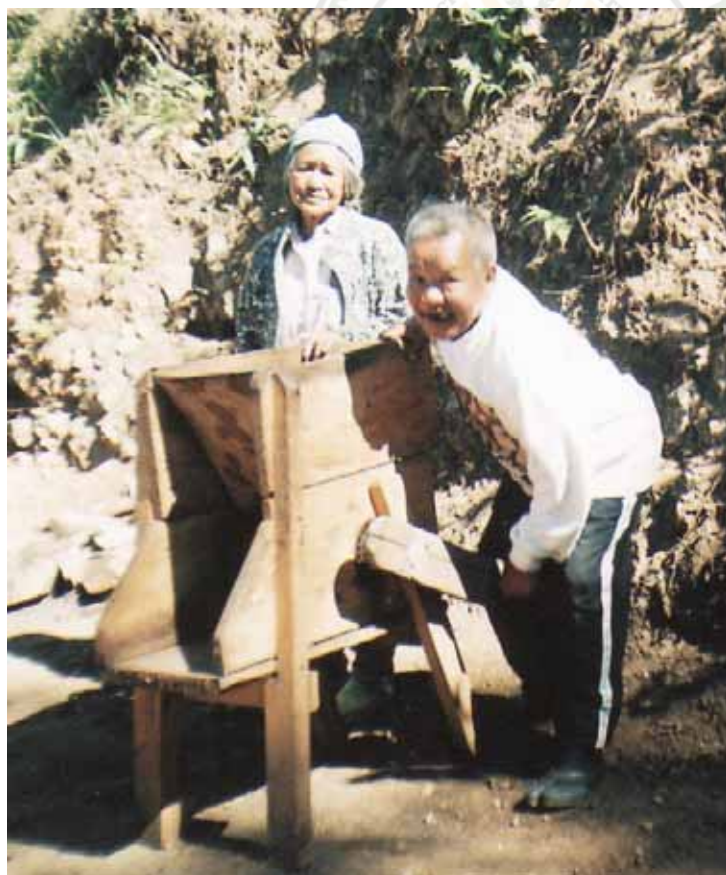
The coffee farmers with the wooden pulper that is used in pulping the coffees that was harvested.
