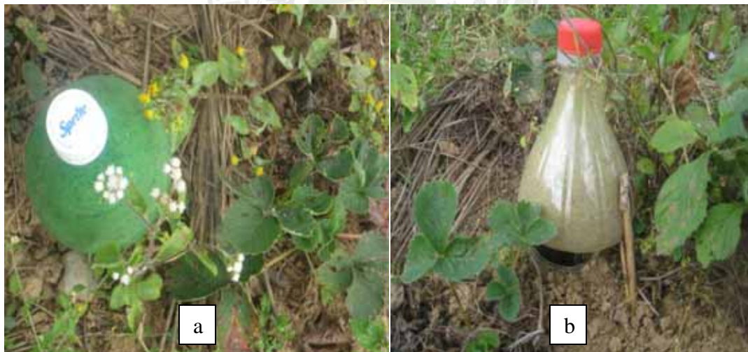
Figure 4. Improved Pitfall trap cover. a.) Top view and b.) Side view
