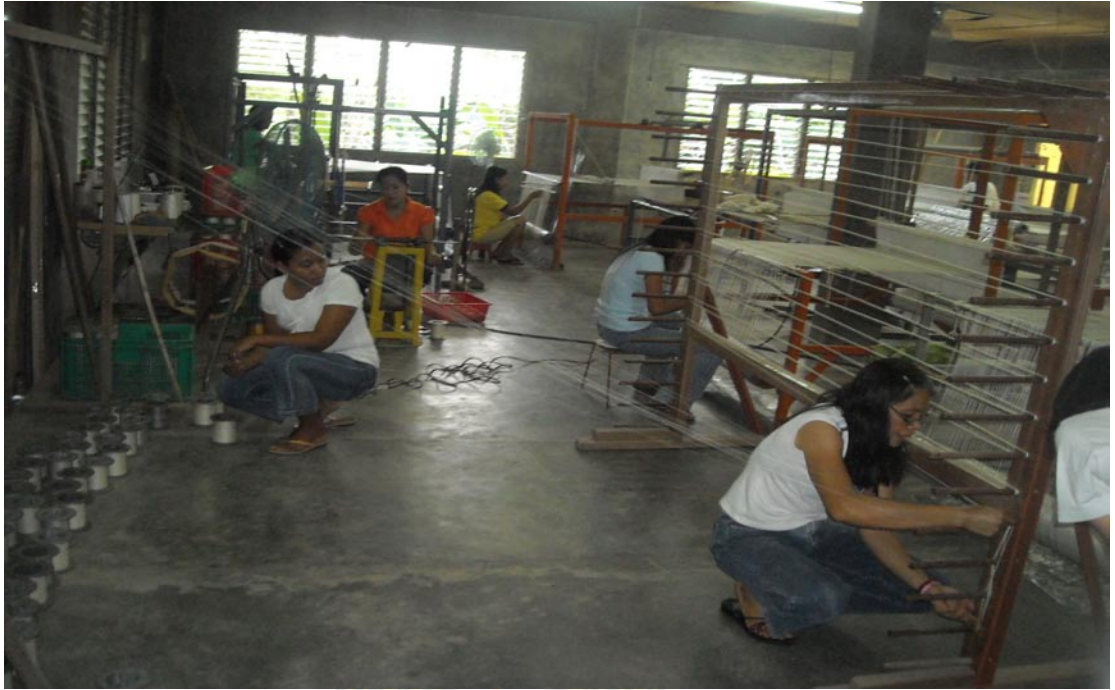
Figure 8. Measuring the length of the warp to be used in weaving to minimize the waste of thread, SRDI filature, January 2010
