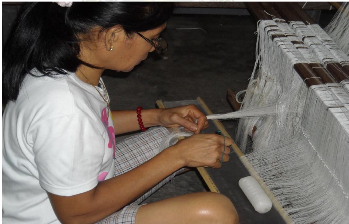
Figure 9. Tying the loam warp ends before weaving, SRDI filature, January 2010
