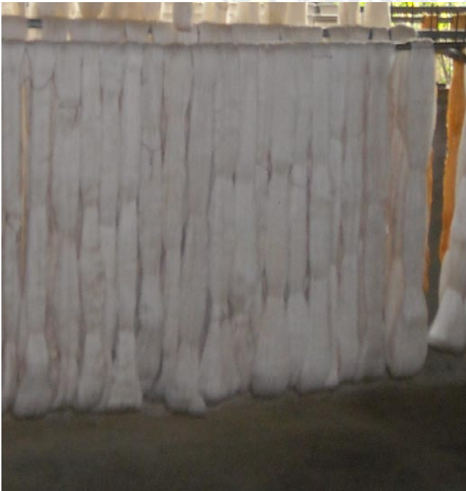
Figure 12. Raw silk laced and hanged to be air dried. Raw silk will go through a series of operations which condition the thread before it is woven into fabric
