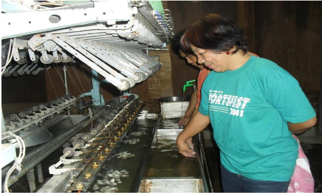
Figure 6. Reeling or the unwinding process of the silk filament from the cocoons, SRDI filature, January 2010
