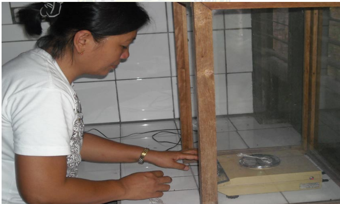
Figure 5. Size filament testing of cocoons before reeling to determine the number of cocoons to be reeled into single thread of required denier, SRDI filature, January 2010
