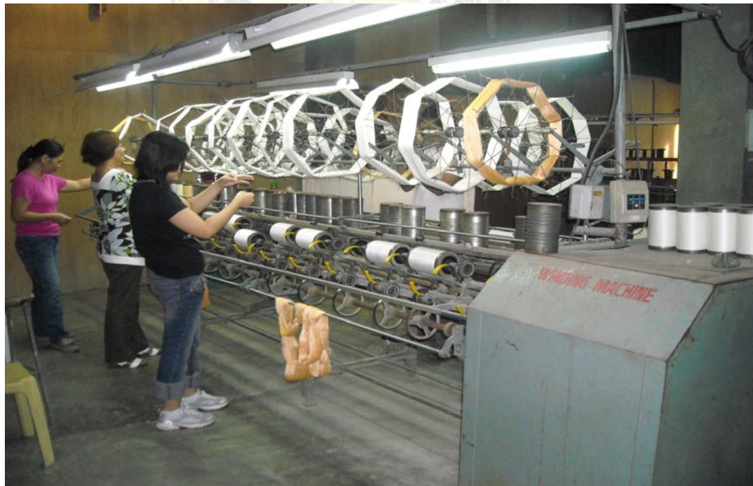
Figure 7. Transferring of raw silk into winding bobbins to facilitate the subsequent processes, SRDI filature, January 2010
