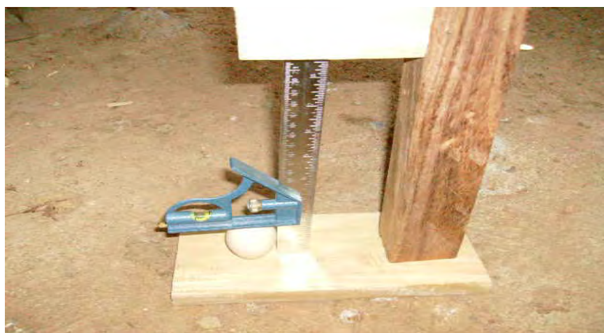
Figure 5. Multi-square used to measure egg length and diameter
