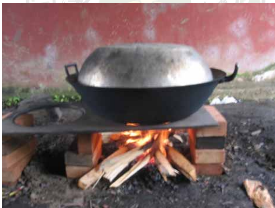
Figure 17. Low Power Boiling Test (metal plate stove)
