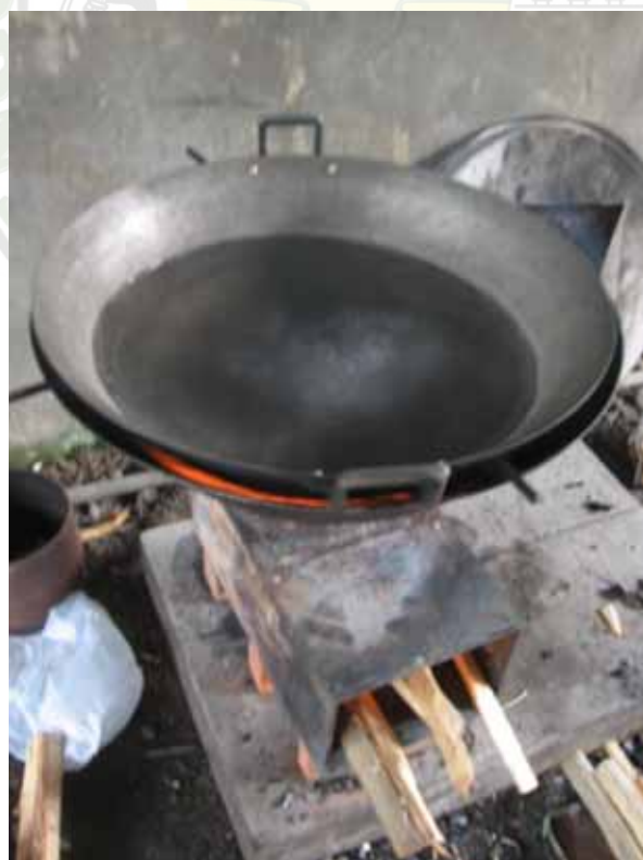
Figure 13. High Power Boiling Test (height 1)
