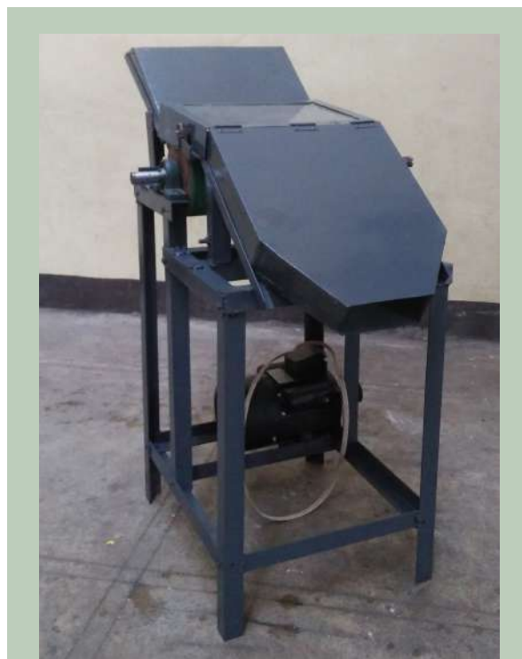
Figure 5. The motorized cocoon deflossing machine
