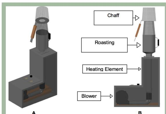
Figure 1. Isometric (A) and front view (B) of roaster
