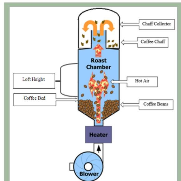
Figure 2. Schematic diagram of the roasting principle in the machine
