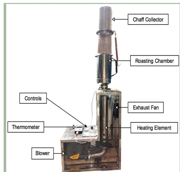
Figure 3. Overview of the batch - type fluidized bed coffee roaster designed in the study.
