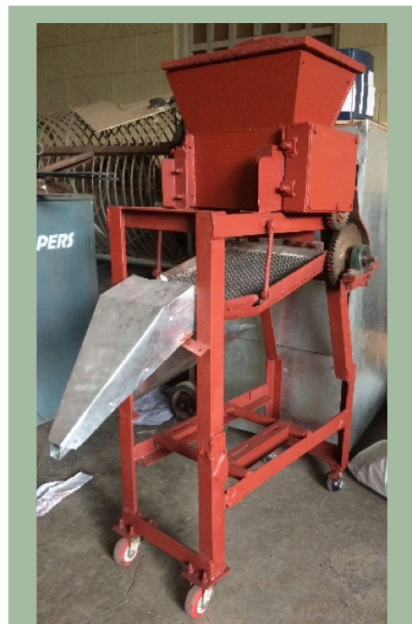
Figure 6. The designed and fabricated oyster shell crusher machine
