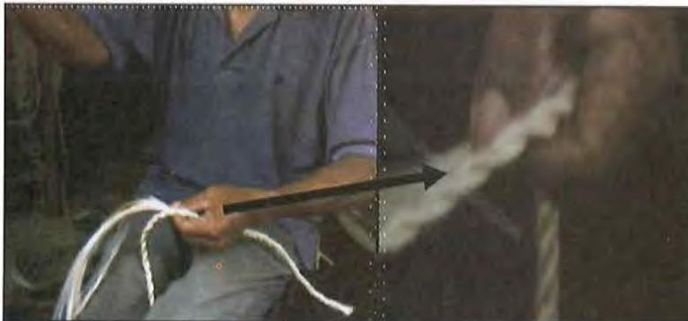
**Step 9.** While twisting, the clustered strands are alternately connected to make the desired length of the twine rope. The twines can be twisted by hand or with a use of improvised tools/ simple machine.
