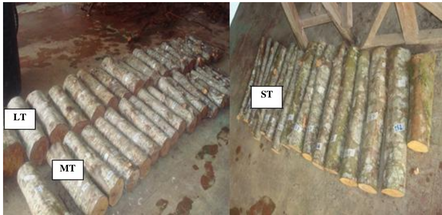
Figure 4. Logs cut into 0.5 m sections of the selected Alnus trees: LT – large tree, MT – medium tree, and ST – small tree
